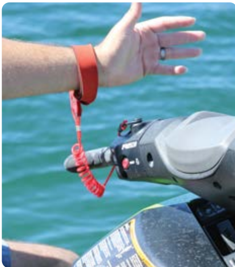
A kill switch lanyard attached to your arm stops the engine if you fall overboard.
